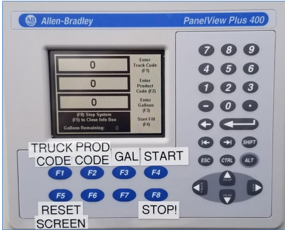
Figure 1: Control Panel for Liquid Loading
